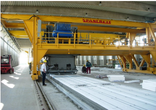
GT-240 system producing 2.4 meter wide insulated wall panels.
