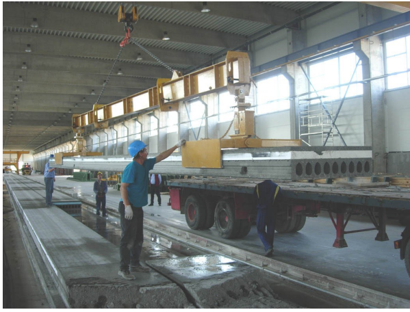
Spancrete GT-240 machinery operating in Hevesbeton Kft. in Hungary Hevesbeton Kft., H-3360 HEVES, Arany J. u. 62., Hungary
