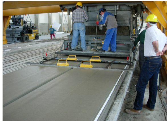
Production of “Divided” Insulated Wall Panels (2, 1.2 Meter panels) with architectural finish.
